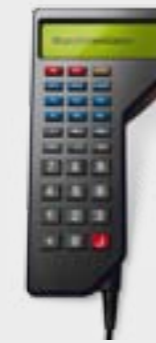
MDE device for detecting the current machine data
